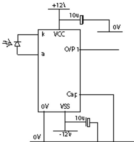
Ambient Light Compensated Modulated Detector
